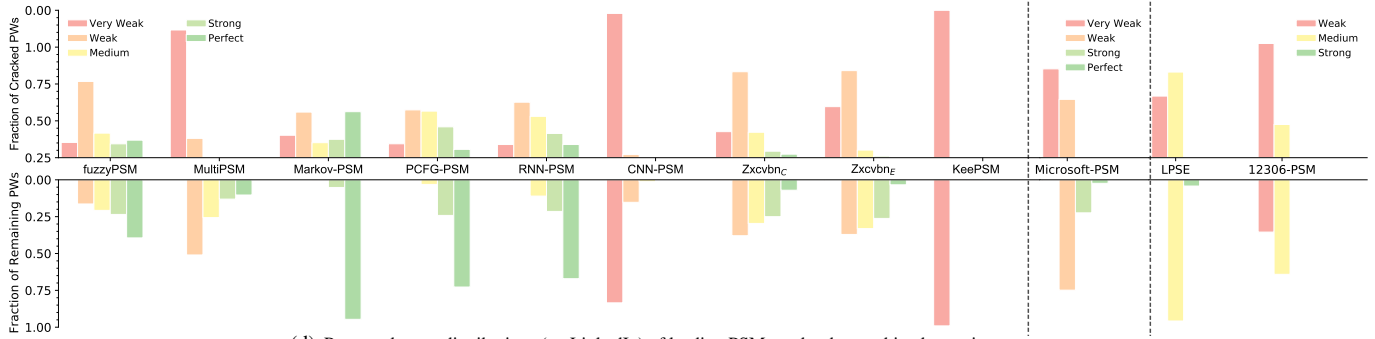
(d) Password score distributions (on LinkedIn) of leading PSMs under the combined guessing strategy.
