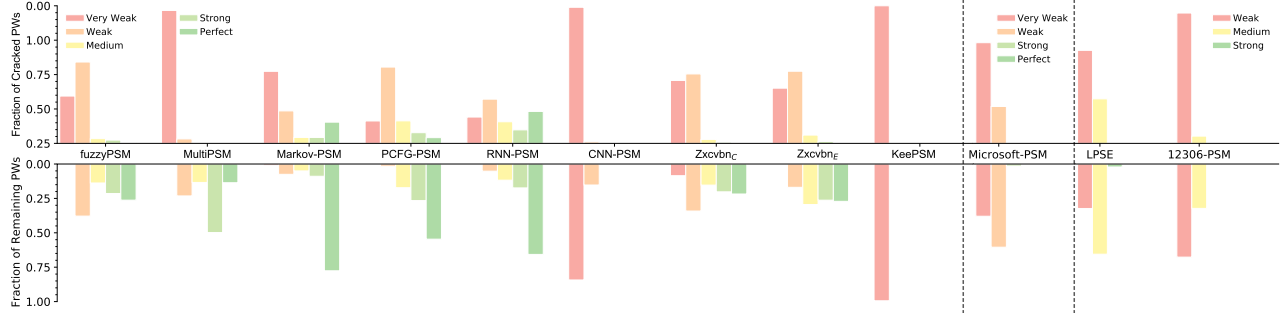
Figure 5: Password score distributions (on Weibo) of leading PSMs under the combined guessing strategy. The larger fractions of cracked low-score and remaining high-score passwords indicate a more accurate PSM. For more results under other guessing strategies on Weibo and LinkedIn, see Figs. 14 and 15.
